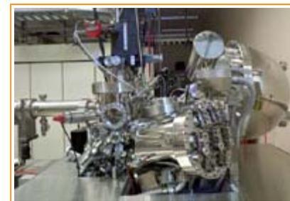
Figure 3. Photoemission Chamber
