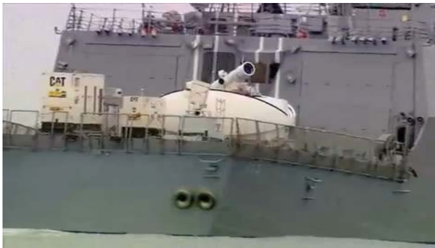
Amazing Navy Laser Weapon System Shoots Down Drone: The Laser Weapon System (LaWS) is a technology demonstrator built by the Naval Sea Systems Command from commercial fiber solid state lasers. LaWS can be directed onto targets from the radar track obtained from a MK 15 Phalanx Close-In Weapon system.
