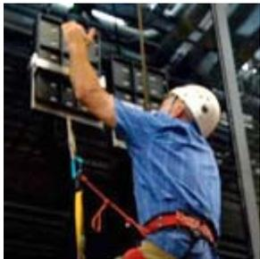
DARPA's Z-Man program has demonstrated the first known human climbing of a glass wall using climbing devices inspired by geckos. The historic ascent involved a 218-pound climber ascending and descending 25 feet of glass, while also carrying an additional 50-pound load in one trial, with no climbing equipment other than a pair of hand-held, gecko-inspired paddles. The novel polymer microstructure technology used in those paddles was developed for DARPA by Draper Laboratory of Cambridge, Mass.
