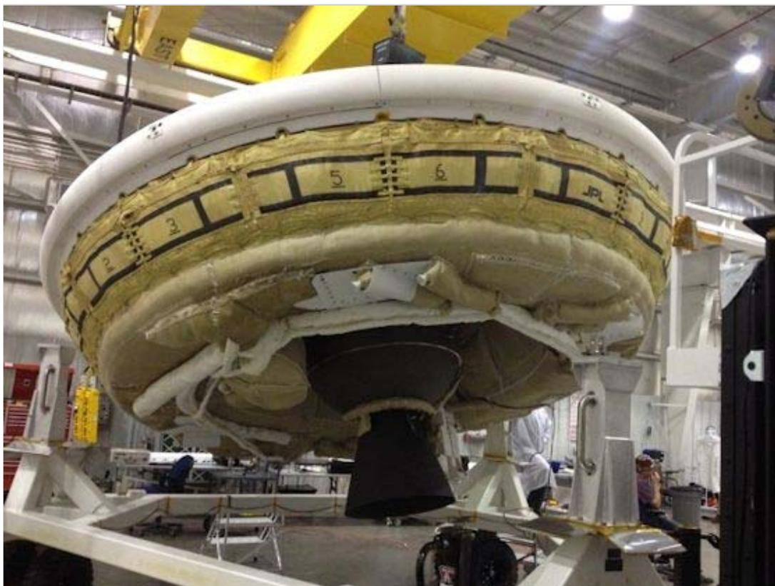
A saucer-shaped test vehicle holding equipment for landing large payloads on Mars is shown in the Missile Assembly Building at the US Navy's Pacific Missile Range Facility in Kaua'i, Hawaii. [More](#)
