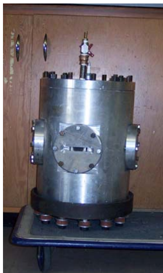
Figure 6.—A 17 liter chamber in which carbon aerosol is gelled.
