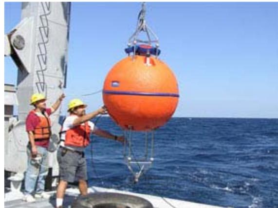
A Long Ranger ADCP housed in a 45 inch in diameter buoyant sphere is launched.
