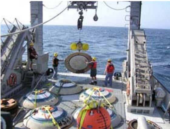
A Barny is launched from the stern of a contract research vessel. A Barny is a trawl-resistant bottom mount that contains an acoustic Doppler current profiler, temperature sensor and pressure gauge.
