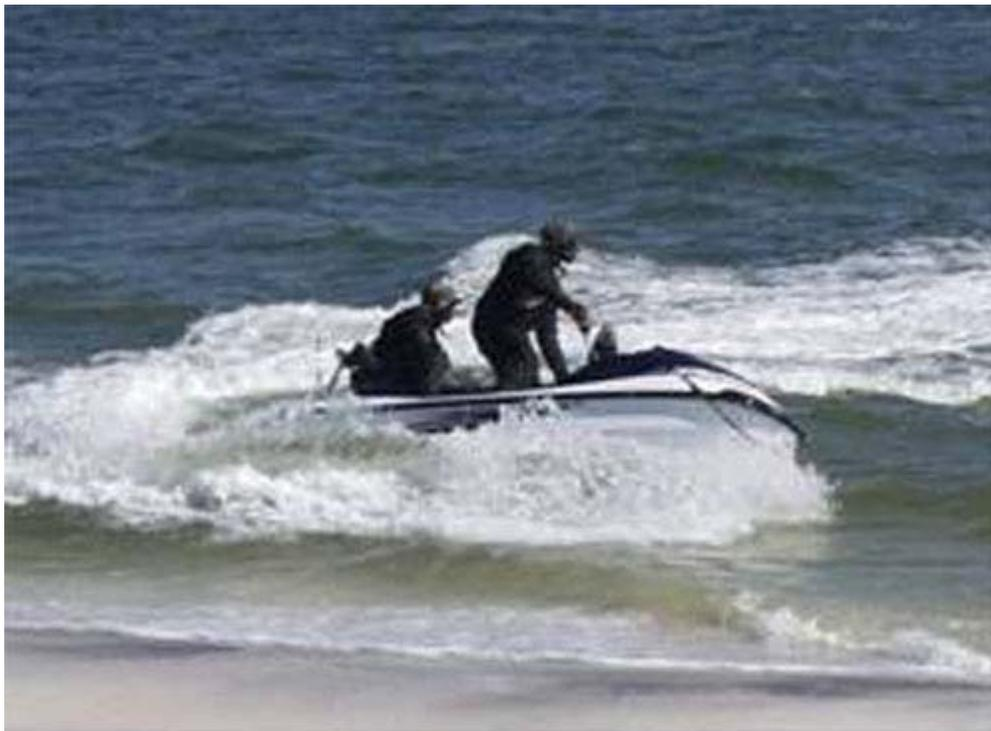
Singlebeam survey conducted from NRL's hydrographic jet ski (Lowrance SBES and Trimble GPS w/ Real Time Kinematic (RTK) base station).
