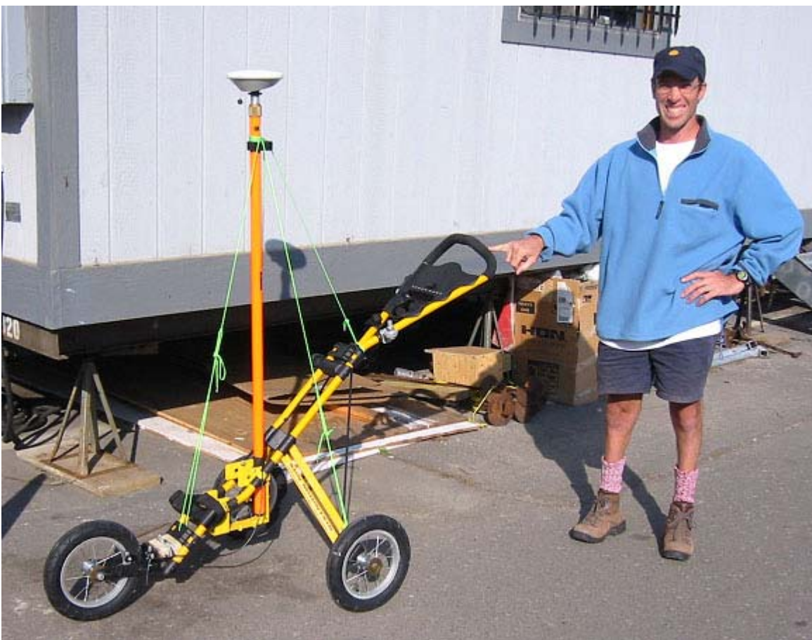
NRL conducted high-resolution surveys using Real Time Kinematic Survey system mounted to this specially-designed vehicle.
