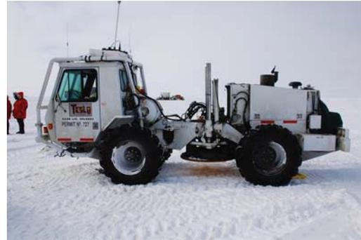
Figure 3: 20,000 lb mini-vibrator (to be modified for tracks).
