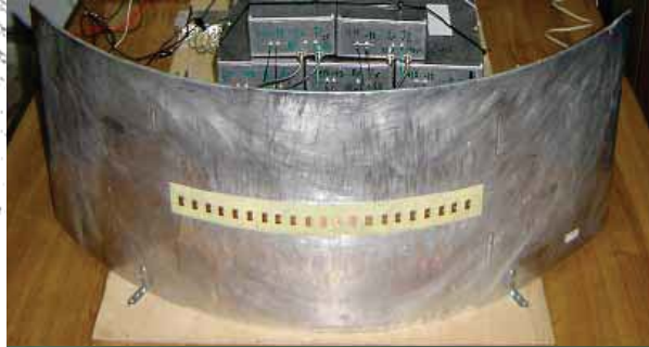
Fig. 1. Cylindrical array test bed antenna.
