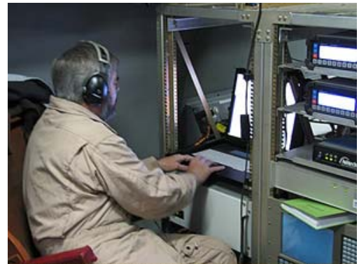
Figure 14. Dr. John Brozena (NRL) closely monitoring Global Positioning System (GPS) and inertial measurement unit (IMU) data to document and resolve deviation from pre-planned flight paths.
