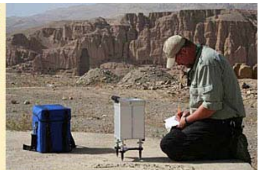
Figure 12. USGS geophysicist Jared Abraham collecting a relative gravity observation in Bamyan, Afghanistan. One of the alcoves that housed a monumental Buddha sculpture (for 1600 years before destruction by the Taliban in 2001) is visible in the background.
