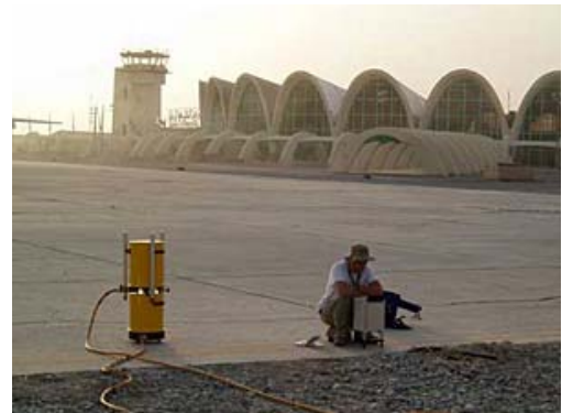
Figure 5. USGS geophysicist Benjamin Drenth collecting a relative gravity observation adjacent to an absolute gravimeter at Kandahar International Airport.
