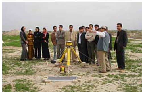
Figure 6. Global Positioning System (GPS) antenna and magnetometer located in Sheberghan, Afghanistan. This temporary base station was maintained and operated by Afghan scientists from the Northern Afghanistan Oil and Gas Exploration Office (Ministry of Mines and Industries).
