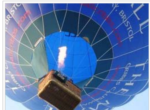
A hot air balloon seen from nearly directly below. The burner flame is firing into the envelope
