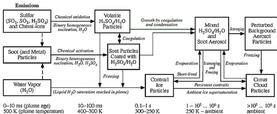
Aerosol and contrail formation processes in an aircraft plume and wake as a function of plume age and temperature. (image courtesy GRID-Arendal)
